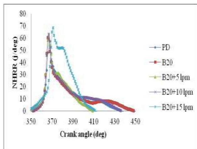
Fig.11: Variation of Net heat release rate with crank angle at 240 bar IOP
