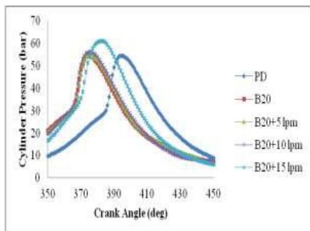
Fig.8: Variation of cylinder pressure with crank angle at 240 bar IOP
