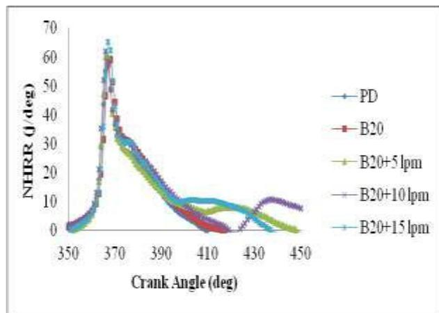
Fig.10: Variation of Net heat release rate with crank angle at 220 bar IOP
