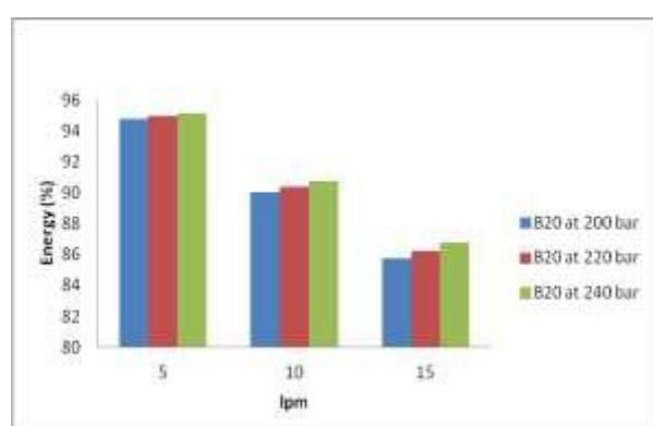
Fig.2: B20 energy share (%) with Hydrogen flow rate (lpm) at different injection operating pressure
