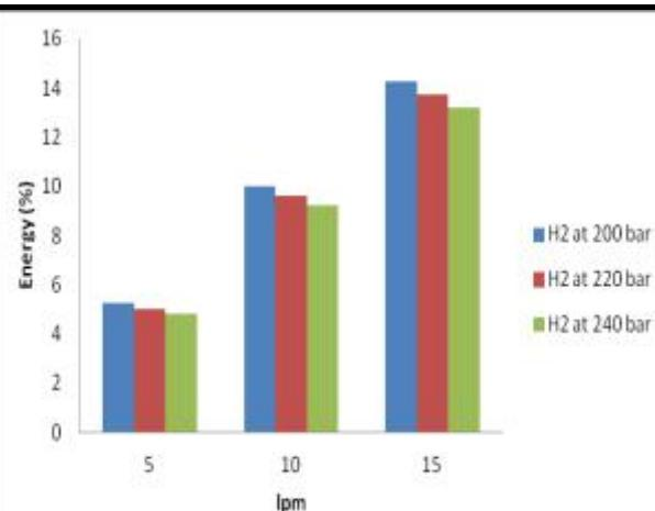
Fig.3: Hydrogen energy share (%) with Hydrogen flow rate (lpm) at different injection operating pressure
