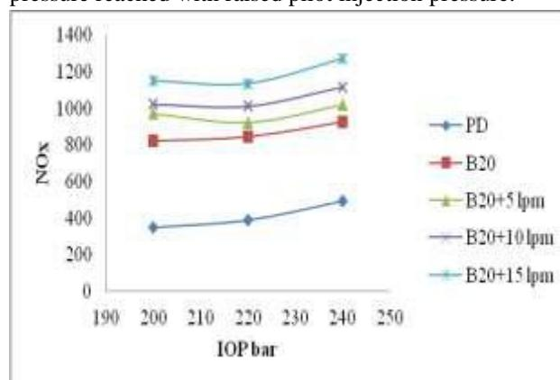
Fig.14: Variation of various NOx emissions with different IOP at 100% load
