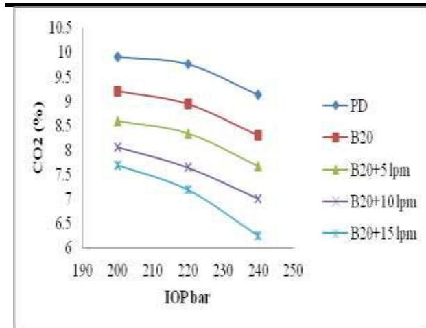
Fig.13: Variation of various CO<sub>2</sub> emissions with different IOP at 100%load
