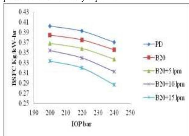
Fig.5: Variation of Brake Specific Fuel Consumption With different Injection Operating Pressure at 100% load
