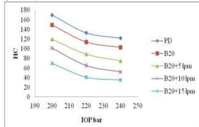
Fig.15: Variation of HC emissions with different IOP at 100 % load
