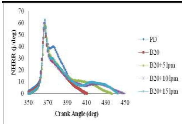
Fig.9: Variation of Net heat release rate with crank angle at 200 bar IOP
