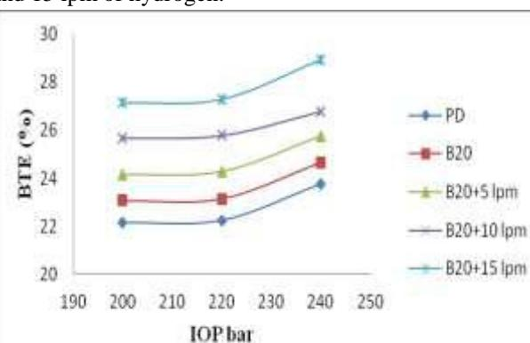
Fig.4: Variation Brake Thermal Efficiency with IOP with 100% load
