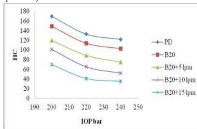
Fig.15: Variation of HC emissions with different IOP at 100 % load
