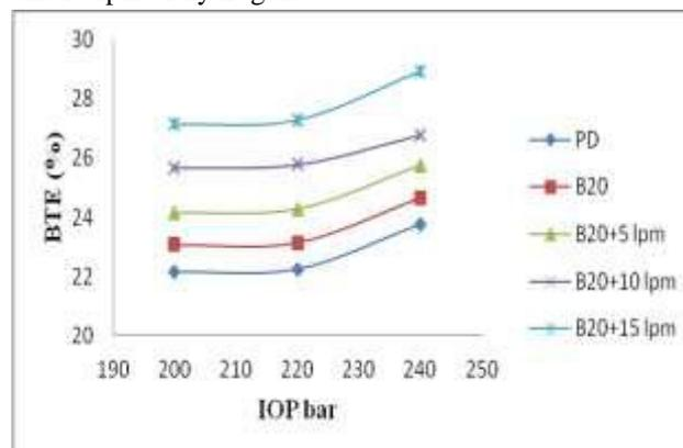
Fig.4: Variation Brake Thermal Efficiency with IOP with 100% load
