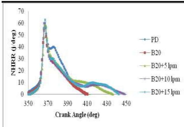
Fig.9: Variation of Net heat release rate with crank angle at 200 bar IOP
