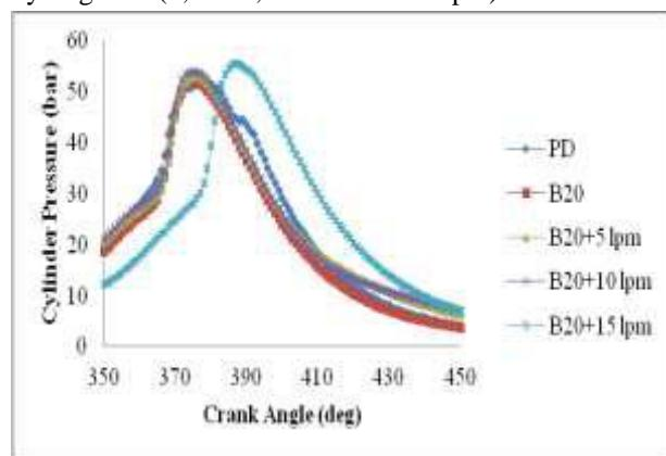
Fig.6: Variation of cylinder pressure with crank angle at 200 bar IOP
