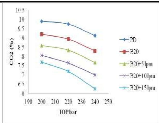
Fig.13: Variation of various CO2 emissions with different IOP at 100% load
