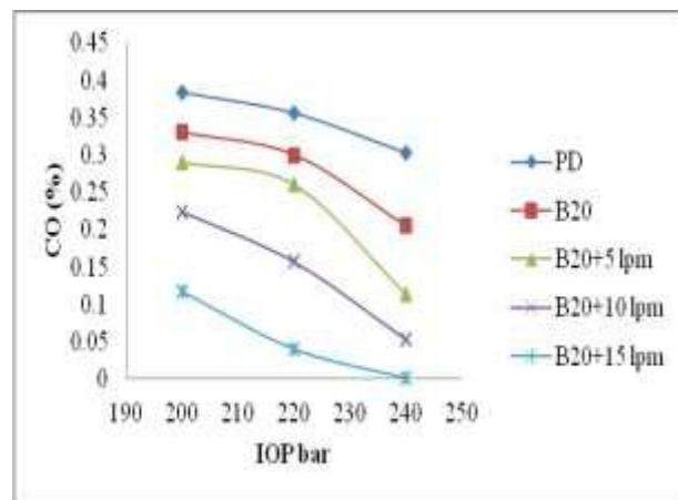
Fig.12: Variation of various CO emissions with different IOP at 100% load
