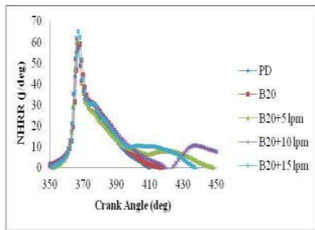
Fig.10: Variation of Net heat release rate with crank angle at 220 bar IOP
